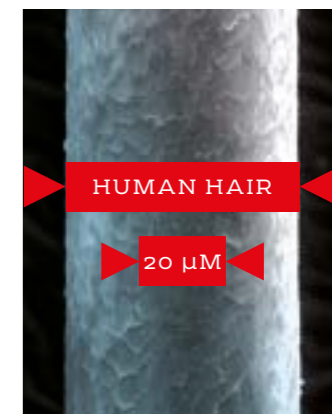
[FIG.20] Comparison between a human hair and the minimum permitted clearance of a con rod bearing of 20 µm.
